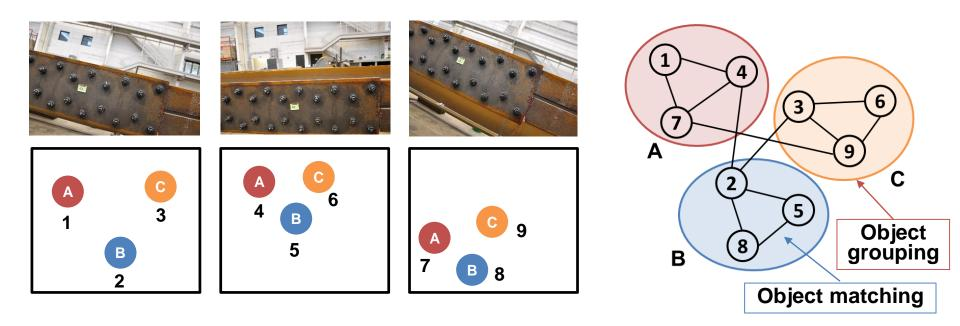
**Object matching:** Integration of SIFT descriptor and epipolar constraint **Object grouping:** Community detection technique (Modularity maximization technique)
